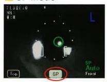
The alignment position for patients with small pupils displays when the SP button is pressed.
